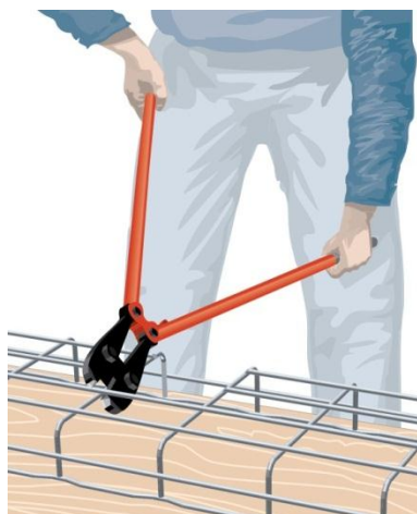
Figure 3-66 Cutting with Bolt Cutters
