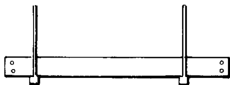
Figure 3-35 Cable Tray Installation
